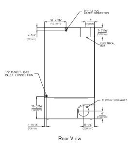
\*Requires 8" (203 mm) material if venting horizontally; 10" (254 mm) if venting vertically. See specific instructions for proper installation.
